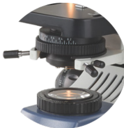
Close-up of graduated Iris diaphragm, graduated Koehler Illuminator diaphragm and graduated fine focus control
