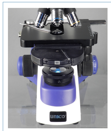
Models with Full-Phase Contrast (10, 40 & 100x S-P Phase Objectives) include the Turret Condenser with positions for 10, 40 & 100x Phase plus a "0" setting for Brightfield objective use and a Centering Telescope to center the condenser with the objectives.
