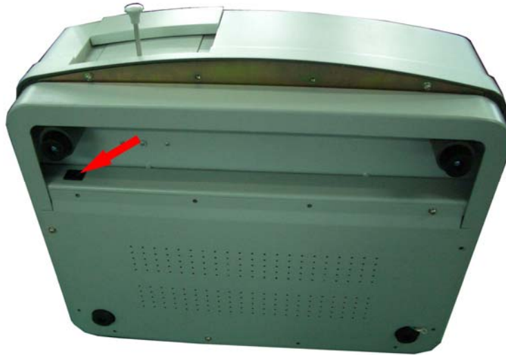
Figure 7.12 Normal/Program Switch for Software Update
