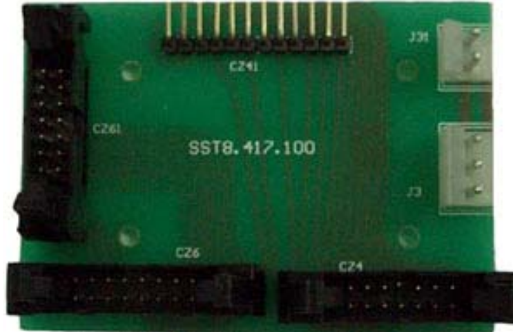
Figure 5.17 Layout of Transferring PCB(In Upper Case)
