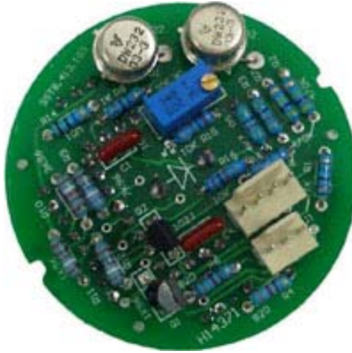
Figure 5.20 Layout of UV-3802 Slave Amplifier PCB
