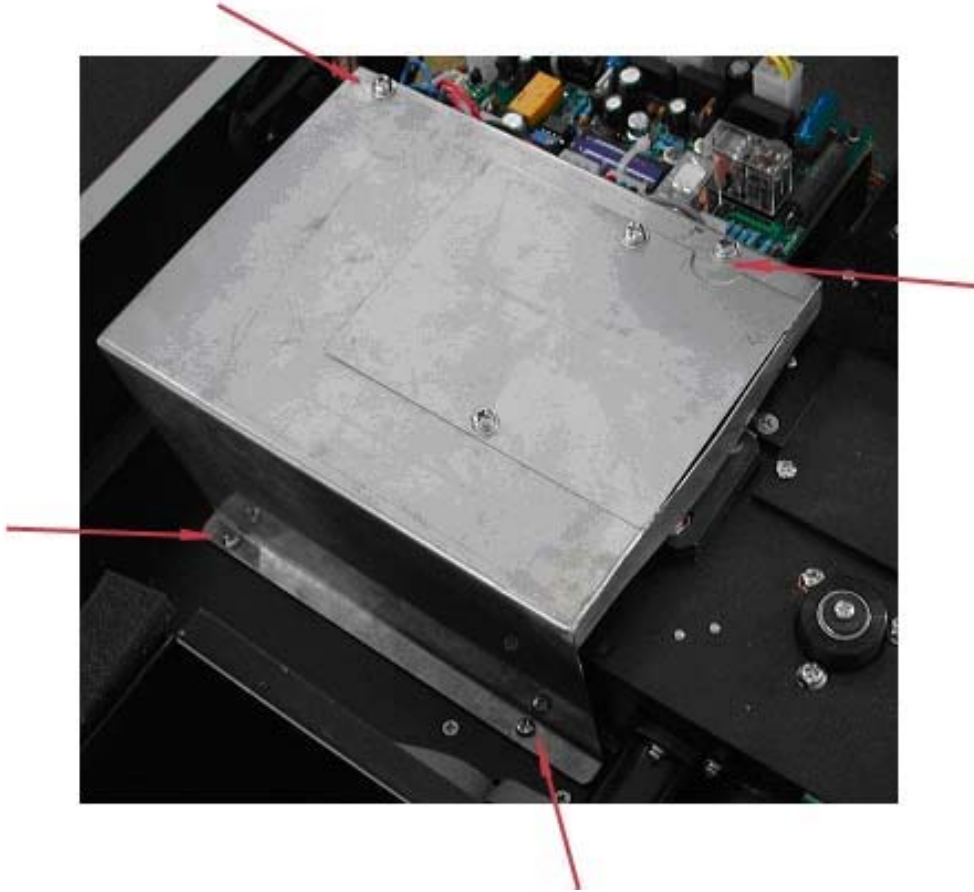
Figure 7.4 Remove the Lamp Cover
