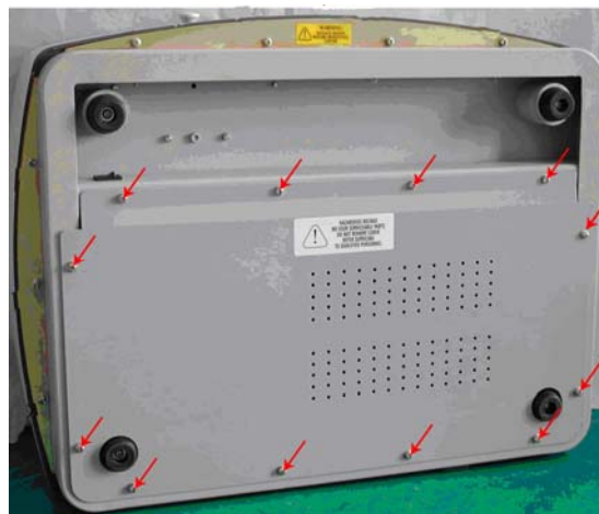
Figure 7. 10 Remove the bottom cover
