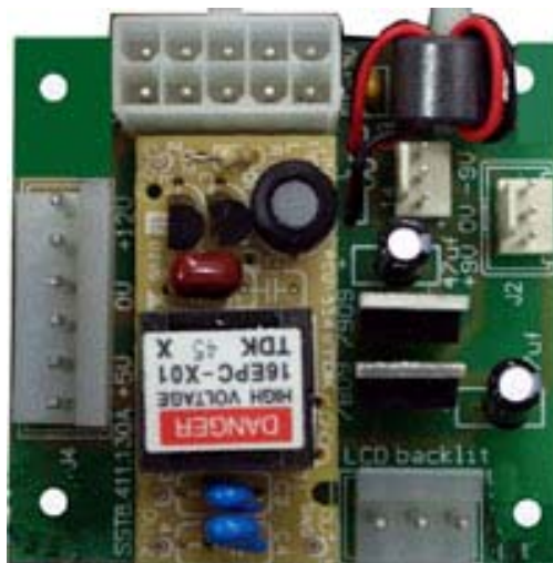
Figure 5.9 Layout of Power Distributing PCB
