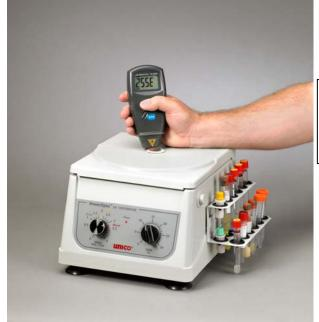
Speed is checked using UNICO digital tachometer. Order part# C800-75
