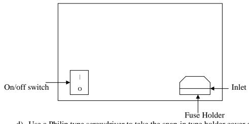
d) Use a Philip type screwdriver to take the snap-in type holder cover off. Remove the blown fuse and replace it with the same type and rating fuse which is:
