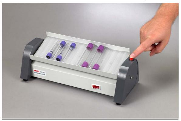
When unloading the specimen push the RED PAUSE button as shown above.
