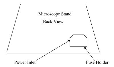
d) Use a flat head type screwdriver to take the snap-in type holder cover off. Remove the blown fuse and replace it with the same type and rating fuse which is:
