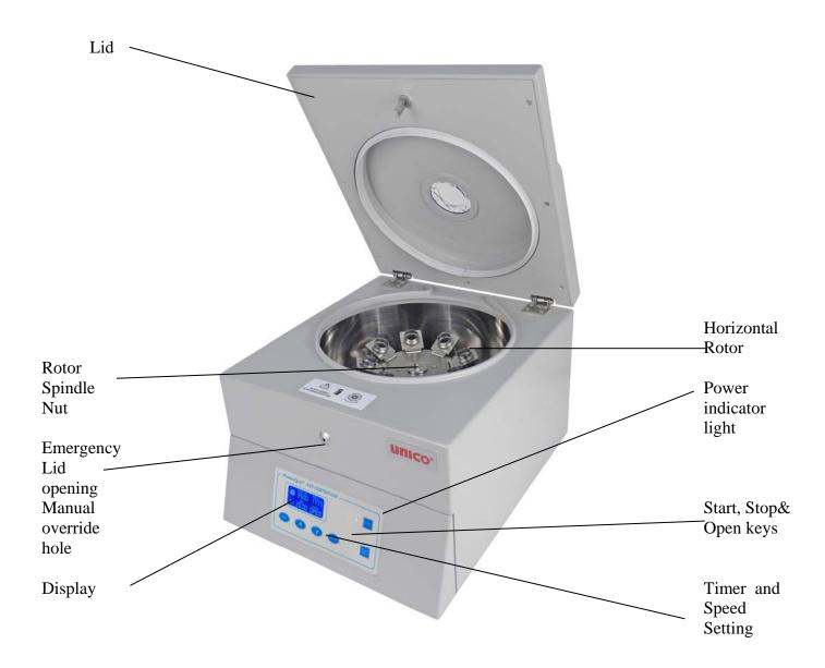
HXV (with 8-place rotor shown) Horizontal Spin Centrifuge
