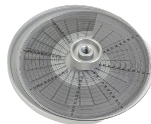
24-position rotor for microhematocrit capillary tubes. Hematocrit reader built into the case
