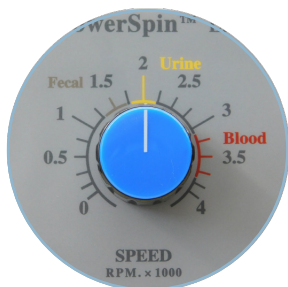
LX color-coded fast speed setting
