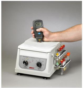
Speed is checked using UNICO digital tachometer. Order part# C800-75
