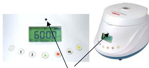
Emergency Opening Hole
