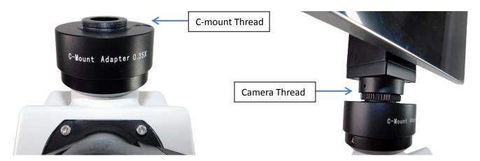
Camera Insertion: Align the camera's threaded connector with the C-mount adapter's threads.
