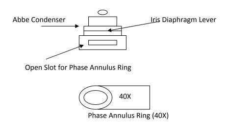
Insert the phase annulus ring all the way down into the slot. Raise the condenser to its highest position by turning the substage knob.
