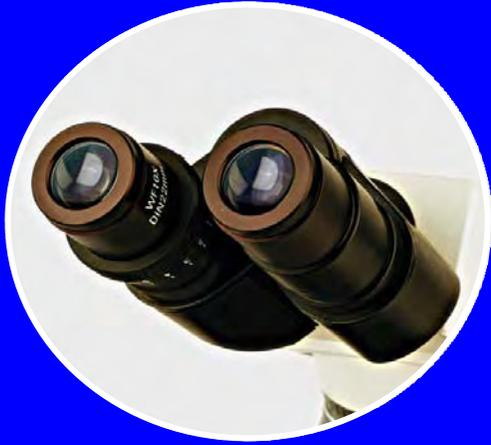
**HEADS:** Available with 30 degree inclined Binocular or Trinocular heads. Featuring Seidentopf optical design with 55 – 75 mm interpupillary distance adjustment. Both heads rotate 360° and lock-in-place with a thumbscrew. One eye tube offers independent focusing diopter adjustment to compensate for the natural vision differential between each eye.
